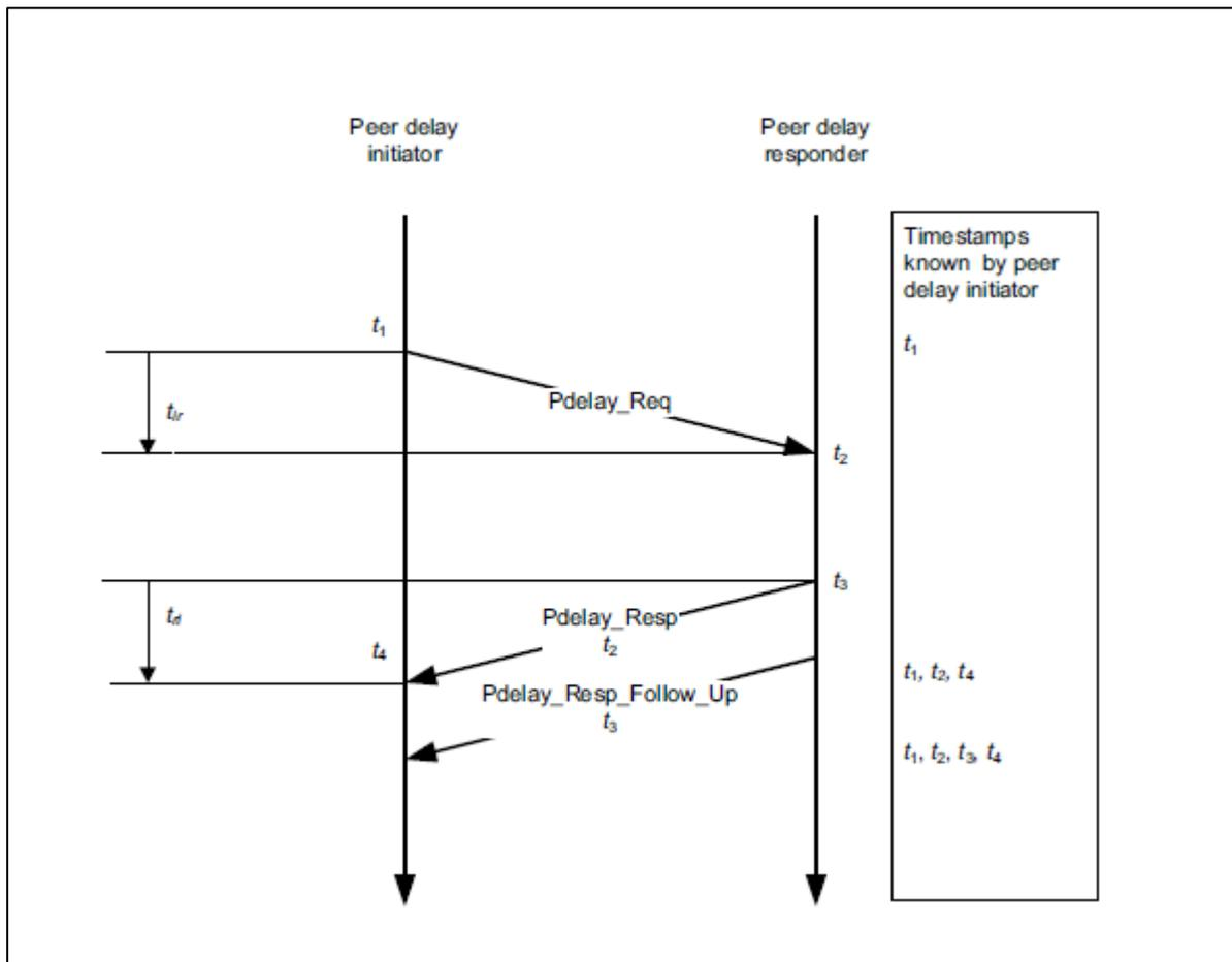
$$D = \frac{t_{ir} + t_{ri}}{2} = \frac{(t_4 - t_1) - (t_3 - t_2)}{2}$$
