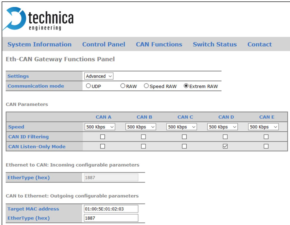
Figure 3-38: Overview CAN Gateway settings in Extreme RAW mode
