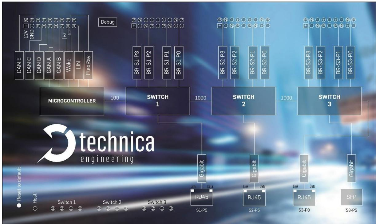
Figure 2-1: Label of MediaGateway with pinning information
